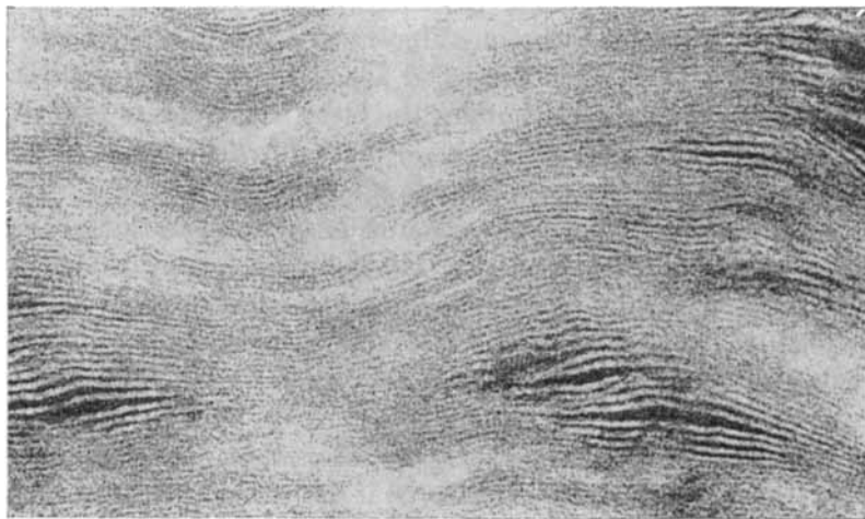
Figure 9. Electron micrograph of potassium oleate gel. c = 81\% , Vestopal embedding, 240 000 : 1.
